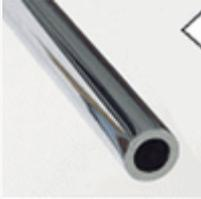
High stress resistance machine-trued hollow steel bars - diameter 16mm - coated with anti-rust chromium-plating. The quality of the materials used adds to the thickness of 2,2mm to prevent the bars from bending: they maintain a perfect shape for a long time. It is possible to choose between the going-through (also called solid) bars and the telescopic type.
